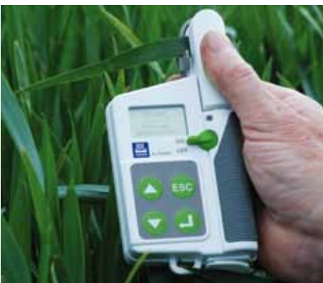
FIGURE 16: The Yara N-Tester is a handheld tool that provides immediate information on actual nitrogen need.
